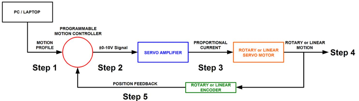
**Step 1.** A program or motion profile will be written on a PC or laptop and downloaded to the motion controller. This program will contain parameters such as speed, acceleration, deceleration, PIDs, desired position, etc...
