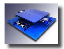
The standard high speed, high acceleration two-axis linear positioning gantry (shown on the left) has a stroke of 8 inches [0.2 meters] (in both the X and Y axes. The force in the X axis is 400 lbs [1780 N] continuous (1200 lb [5340 N] peak) and the force in the Y axis is 200 lbs [890 N] continuous (600 lb [2670 N] peak), although longer strokes and higher forces are available.
