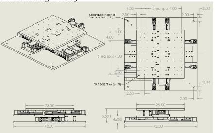
Single-axis Linear Positioning Stage
